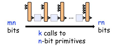
Assuming uniform outputs  $q=\left(2^n\right)^{1-(m-0.5r)/k}$  queries yield a collision w.h.p.
