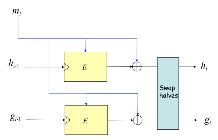
Steinberger recently showed that the iteration of MDC-2 has collision resistance of  $2^{3n/5}$  in the ideal cipher model (concretely,  $2^{74.9}$  for 256 bits of output)
